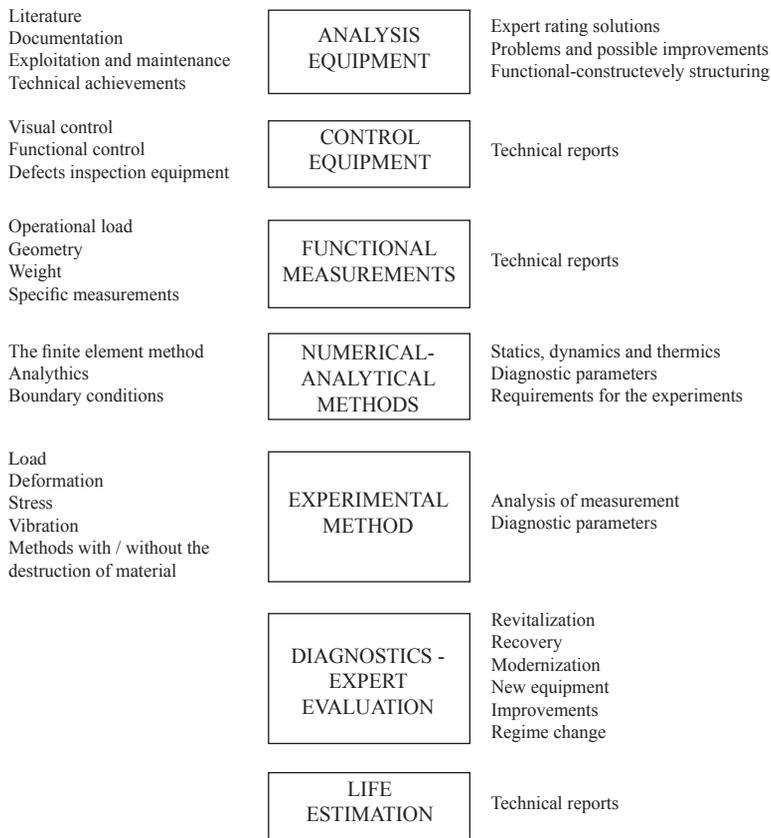
Figure 9 Algorithm for analysis and structure behavior diagnostic
