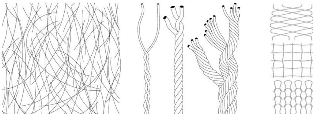
Figure 5. Basic fiber assemblies. With randomly distributed fibers / Figure 6. Basic fiber assemblies. Created by wrapping up. / Figure 7. Advanced fiber assemblies: braided, woven and knitted fibers
