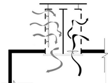
Fig. 8. Adding small fans into traditional wind catcher for increasing the amount of air flow
