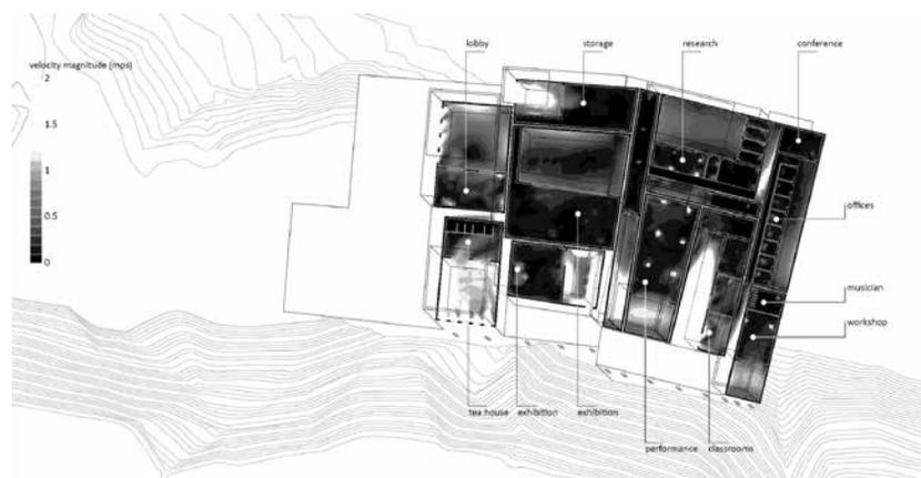
Figure 4. Airflow – computational simulation, Cultural Center in Bamiyan Valley, Afghanistan, conceptual project
